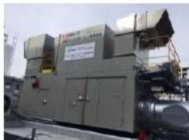
Hydrogen Gas Turbine (1MW class)
